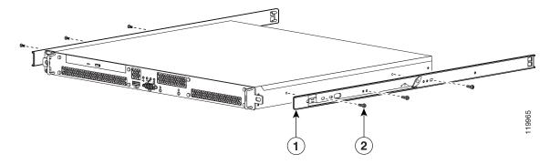
2. Insert the GSS and inner rail into the two outer telescopic rails, as shown in Figure 3-8.
